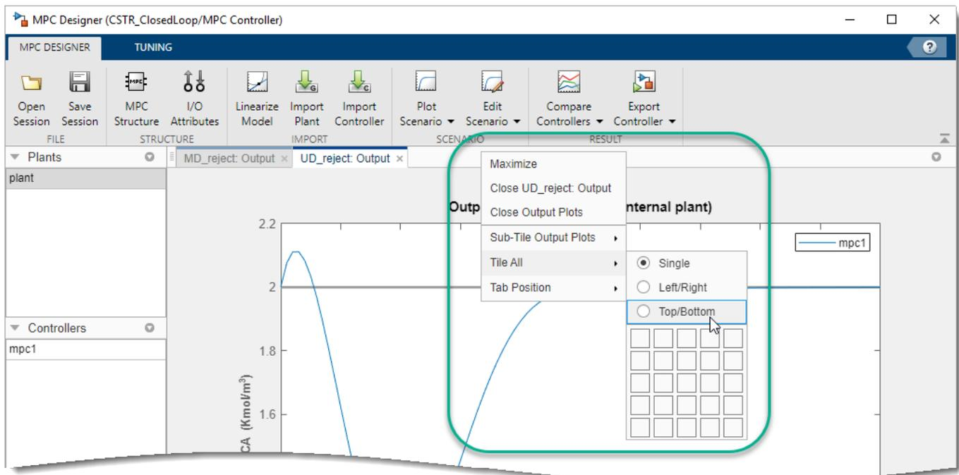
The plot display area changes to display **MD\_reject: Output** tab is in the upper plot area and the **UD\_reject: Output** plot is in the lower plot area.
