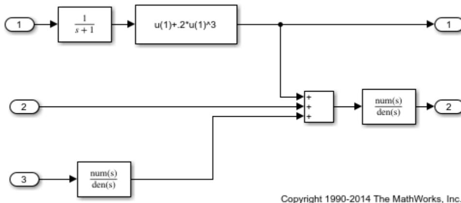
Linearize the plant at the default operating conditions (the initial states of the transfer function blocks are all zero) using the `linearize` command from Simulink® Control Design™.
