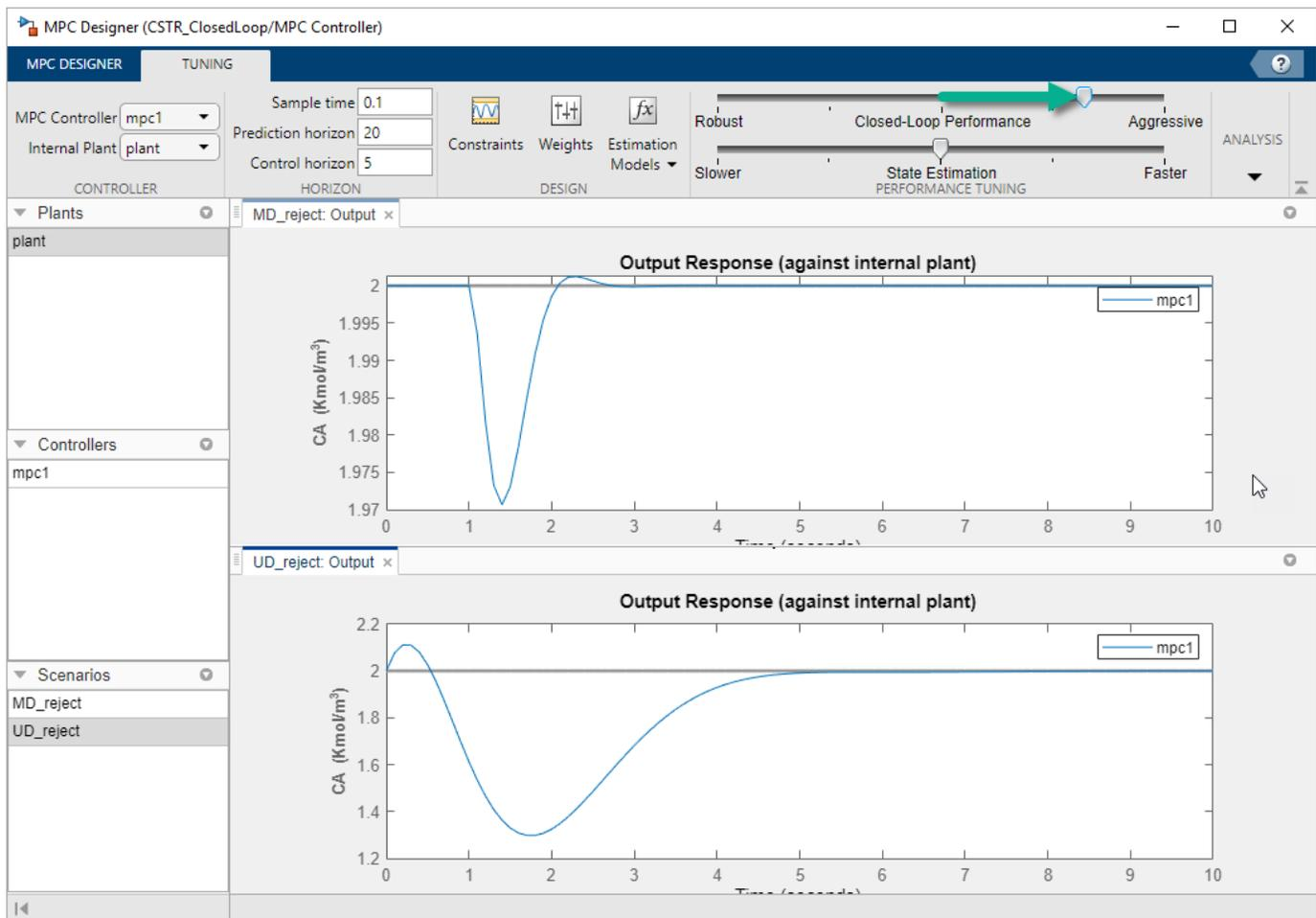
Drag the **State Estimation** slider to the right, which leads to more aggressive unmeasured disturbance rejection. Drag the slider until the **UD\_reject: Output** response reaches steady state in less than 3 seconds.
