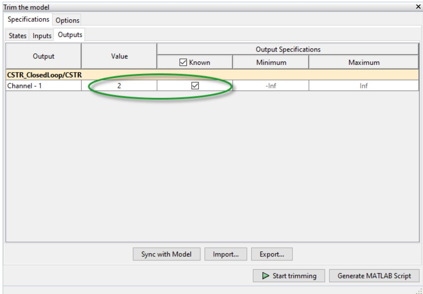
This setting constrains the value of the output signal during the operating point search to a known value.
