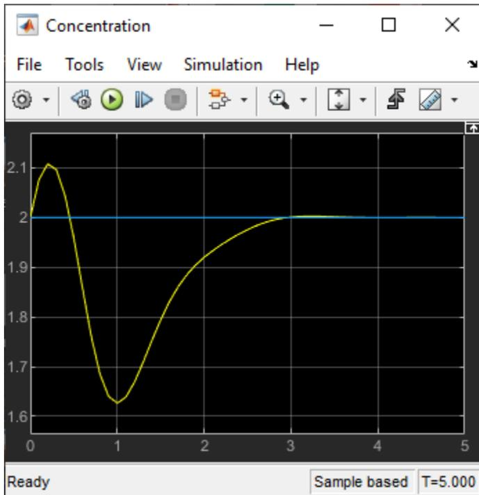
The output response is similar to the **UD\_reject** response, however the settling time is around 1 second longer. The different result is due to the mismatch between the linear plant used in the **MPC Designer** simulation and the nonlinear plant in the Simulink model.
